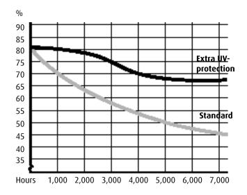
The diagram shows light transmission against time in an accelerated test. 1,000 hours in testing are, very roughly, 2 years of exposure in Scandinavia.
